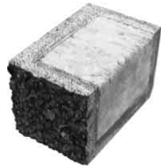
Sample of the material that was used for the façade of Sarphatistraat. In contrast to traditional façades that are made up of a number of layers applied consecutively, we designed a façade consisting of one prefabricated panel that is fitted at once.
